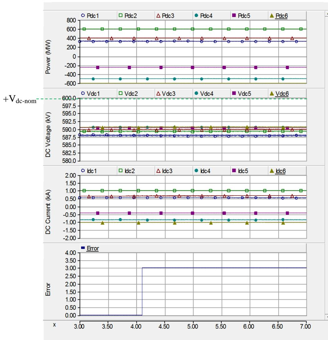
Figure 36: System's response to a DC voltage overload; x-axis is time in seconds.
