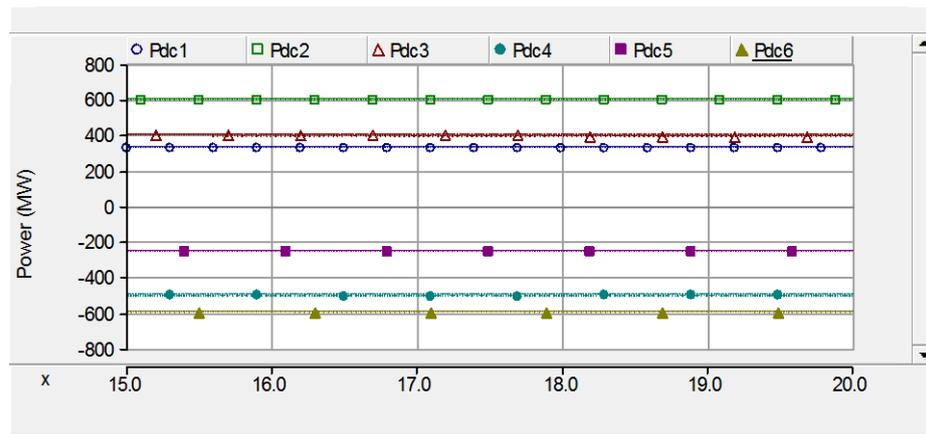
Figure 31: DC power flow at steady-state; x-axis is time in seconds
