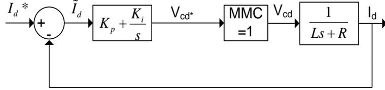
Figure 18: Simplified d-axis current control loop
