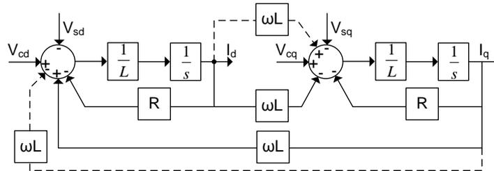
Figure 15: State-block diagram with feedback nulling
