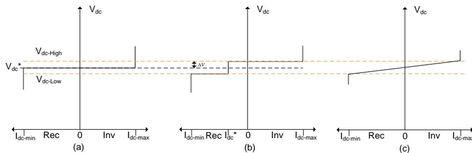
**Figure 23: Typical MT control DC voltage/current characteristics: (a) slack bus; (b) voltage margin; (c) droop**
