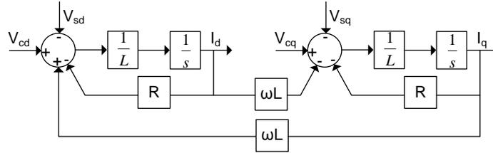
Figure 14: State-block diagram for system plant in dq reference frame
