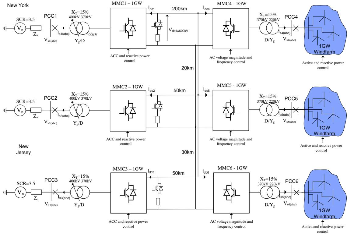
Figure 2: Test model based on the DC configuration for the northern section of the AWC
