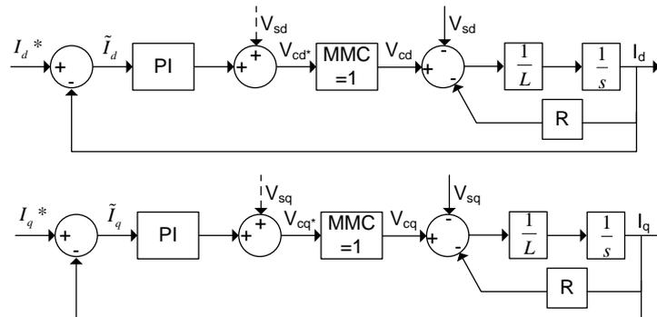
Figure 16: Decoupled d and q current control loops
