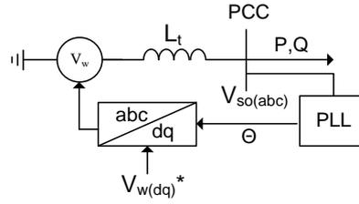
**Figure 28: Implementation of the windfarm power controller**
