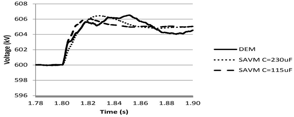
**Figure 20: The models' DC voltage response to a 5kV step change in the DC voltage controller reference voltage at 1.8s.**
