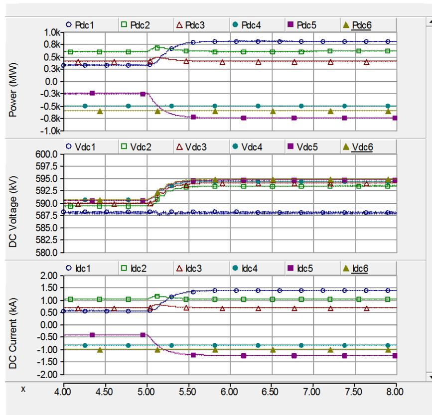
Figure 34: System's response to variations in windfarm power when employing the same droop constant with the PFS engaged using an update frequency of 10; x-axis is time in seconds.
