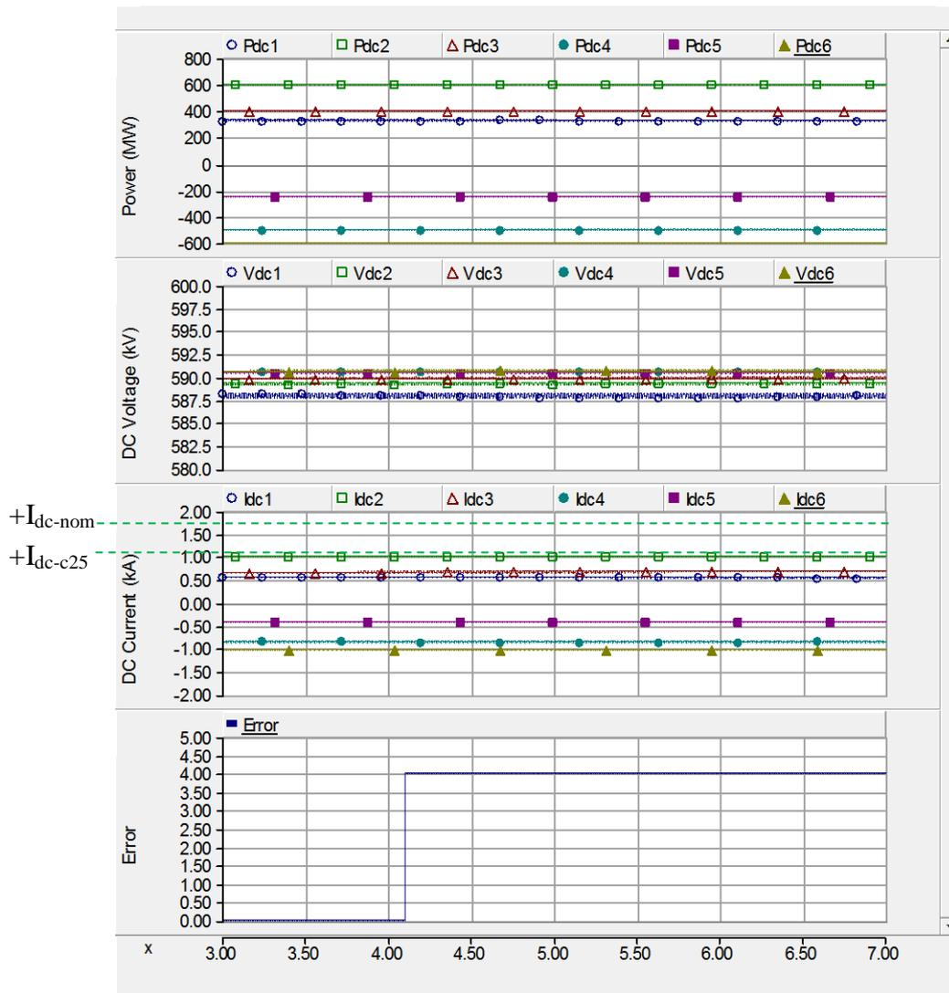
Figure 37: System's response to a cable overcurrent; x-axis is time in seconds.
