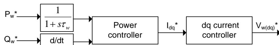
Figure 27: Block diagram for the windfarm power controller
