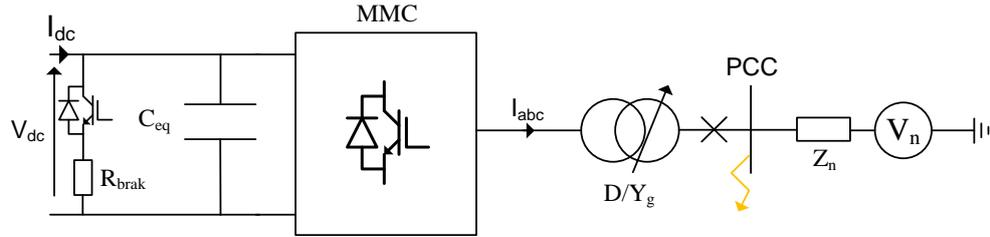
**Figure 6: DC braking resistor**
