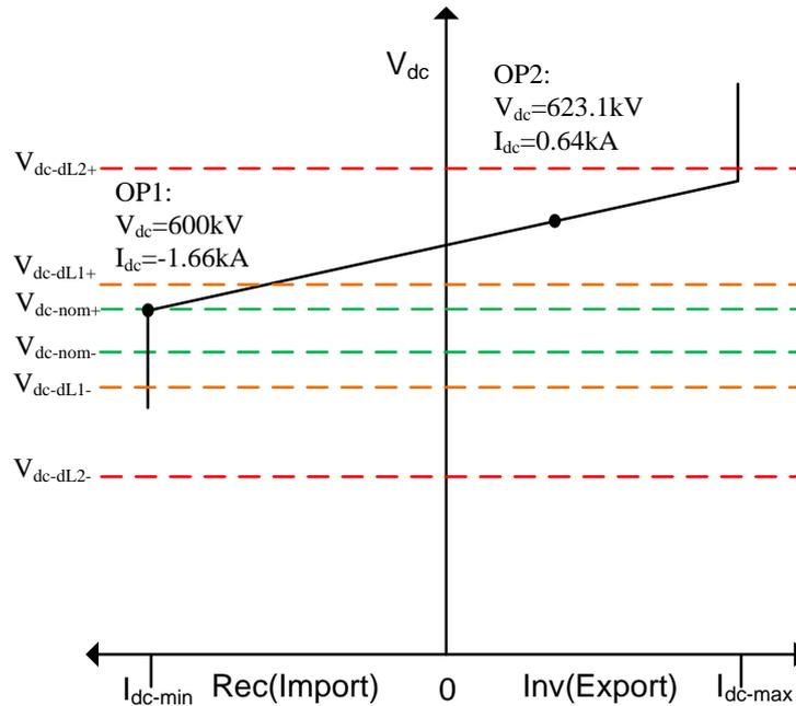
**Figure 29: Operating characteristic for VSC1**
