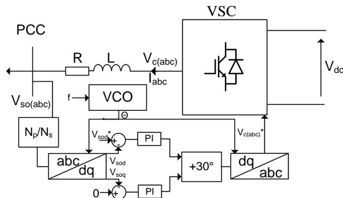
Figure 26: Implementation of the AC voltage controller for the offshore network
