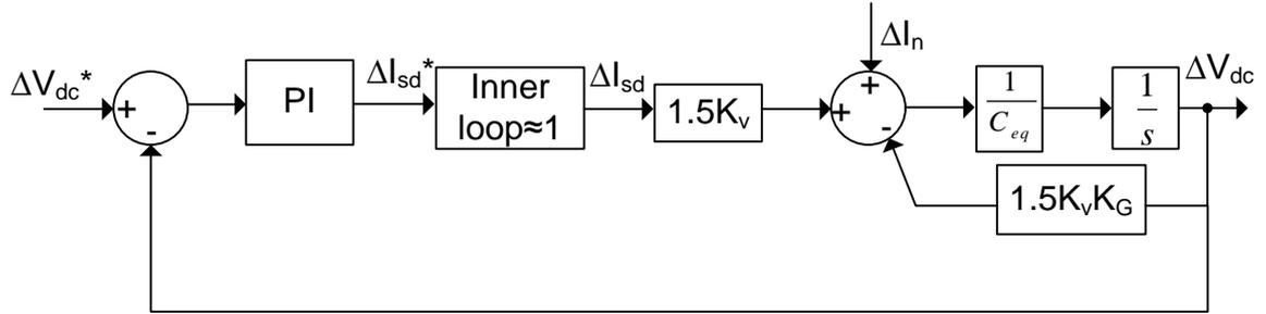
Figure 22: SFSB for DC voltage control loop
