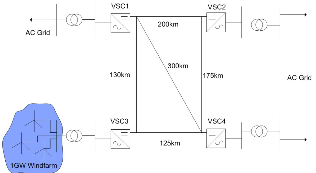
Figure 45: Four terminal PFS test model
