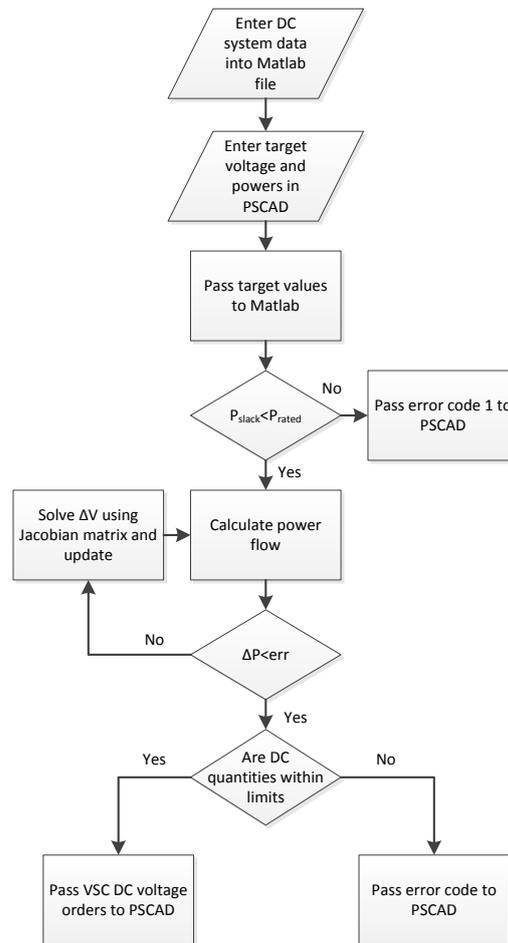
**Figure 10: Flow chart for power flow solver**
