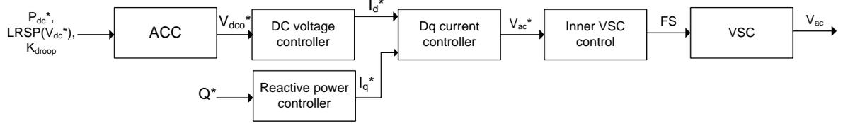
**Figure 24: Basic VSC control structure for ACC**
