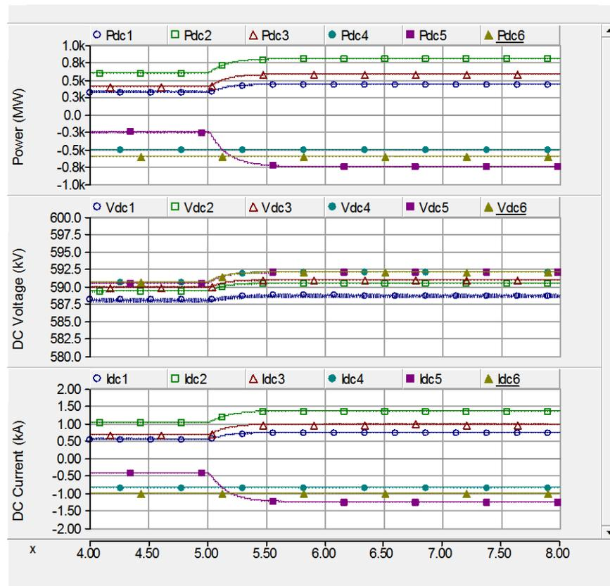
Figure 32: System's response to variations in windfarm power when employing the same droop constant; x-axis is time in seconds
