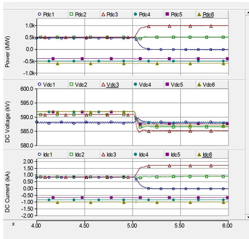
Figure 41: System's response to a power order increase for VSC3 from 500MW to 1000MW at 5s when using the PFS; x-axis is time in seconds.
