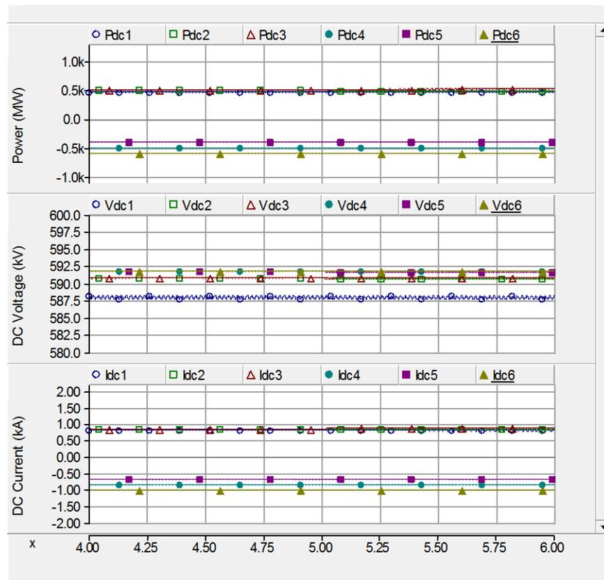
**Figure 44:** System's response to a power order increase for VSC3 from 500MW to 1000MW at 5s without using telecommunications and employing a droop constant of 0.5; x-axis is time in seconds.
