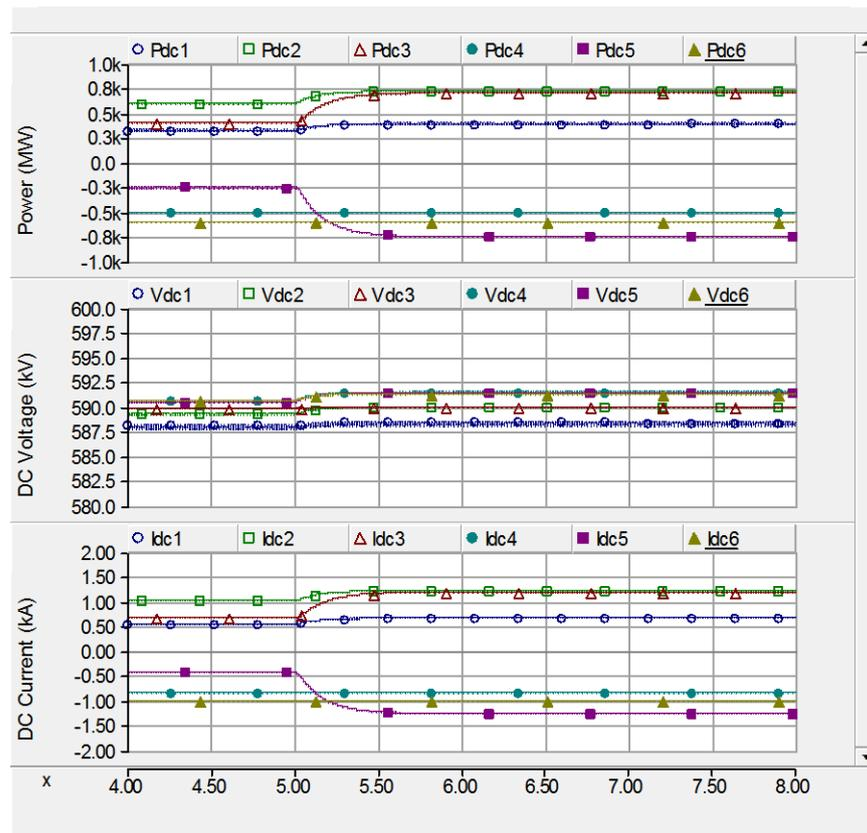
Figure 33: System's response to variations in windfarm power when employing the same droop constant; x-axis is time in seconds
