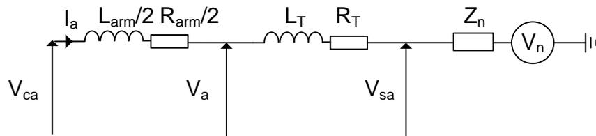
Figure 12: MMC phase A connection to AC system
