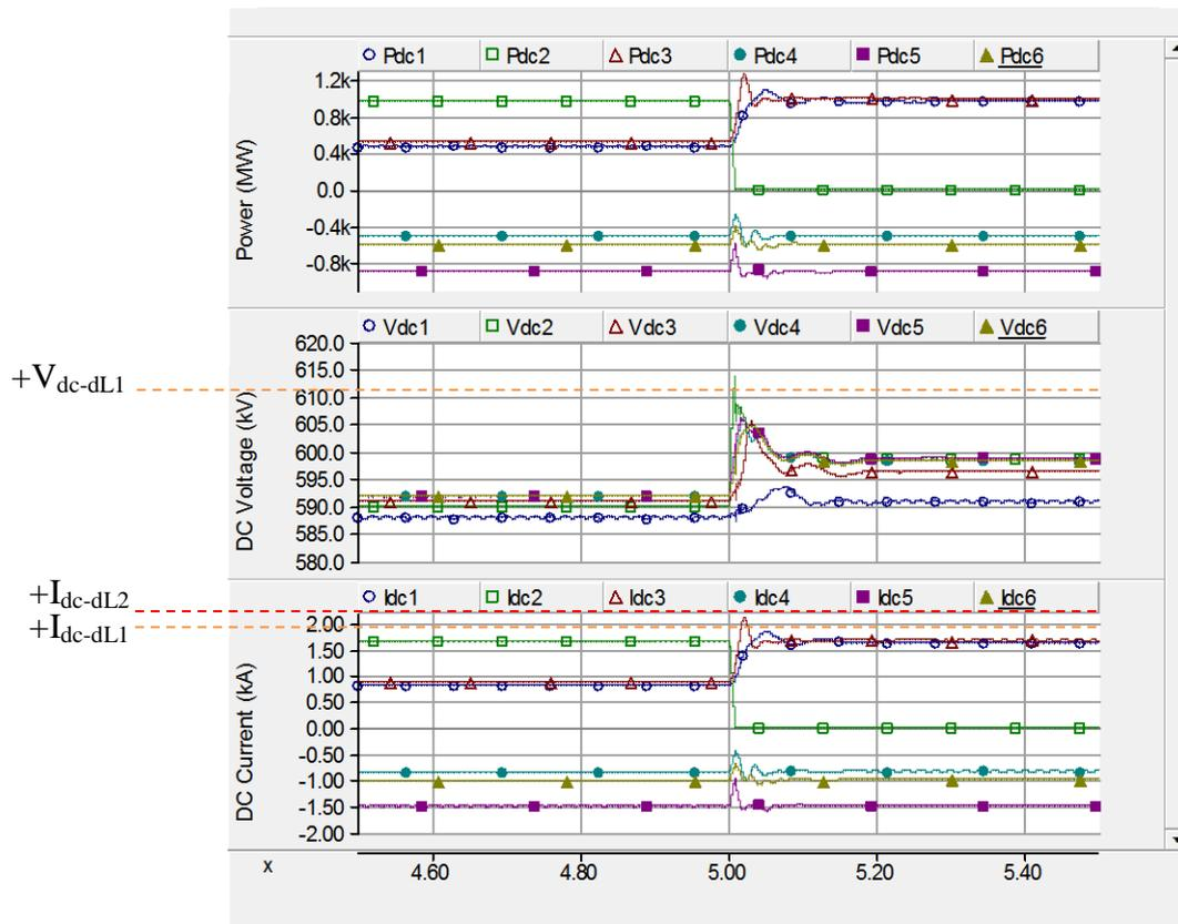
Figure 38: System's response to VSC2 being blocked at 5s; x-axis is time in seconds.
