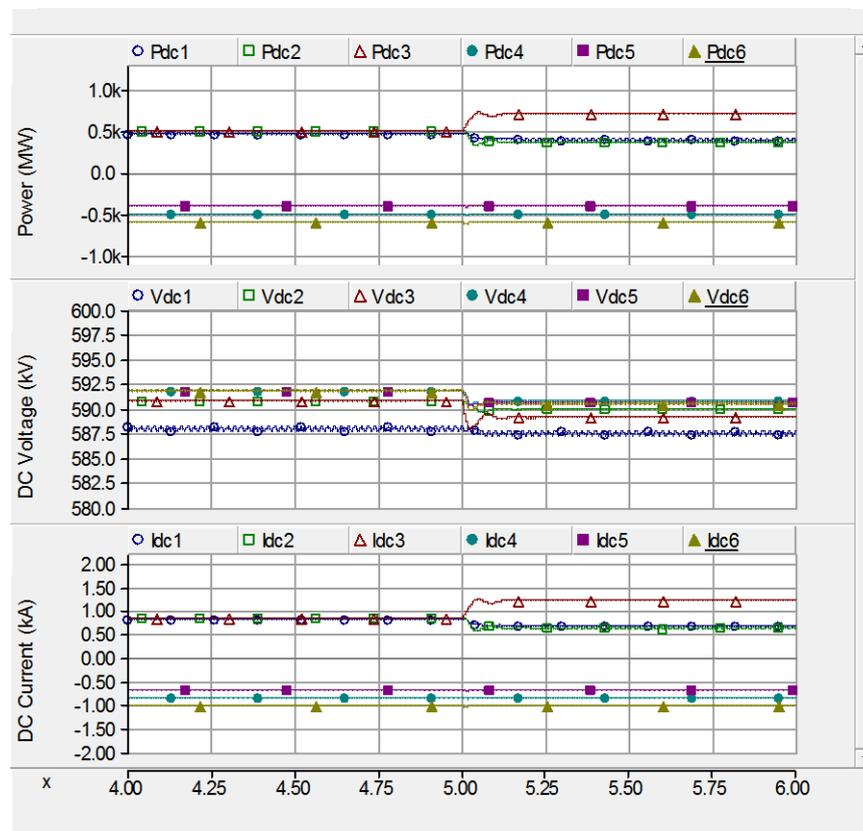
**Figure 43: System's response to a power order increase for VSC3 from 500MW to 1000MW at 5s without using telecommunications; x-axis is time in seconds.**
