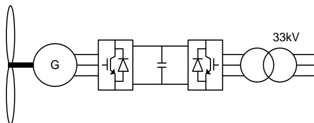
**Figure 7: Simplified diagram of a full scale converter wind turbine**
