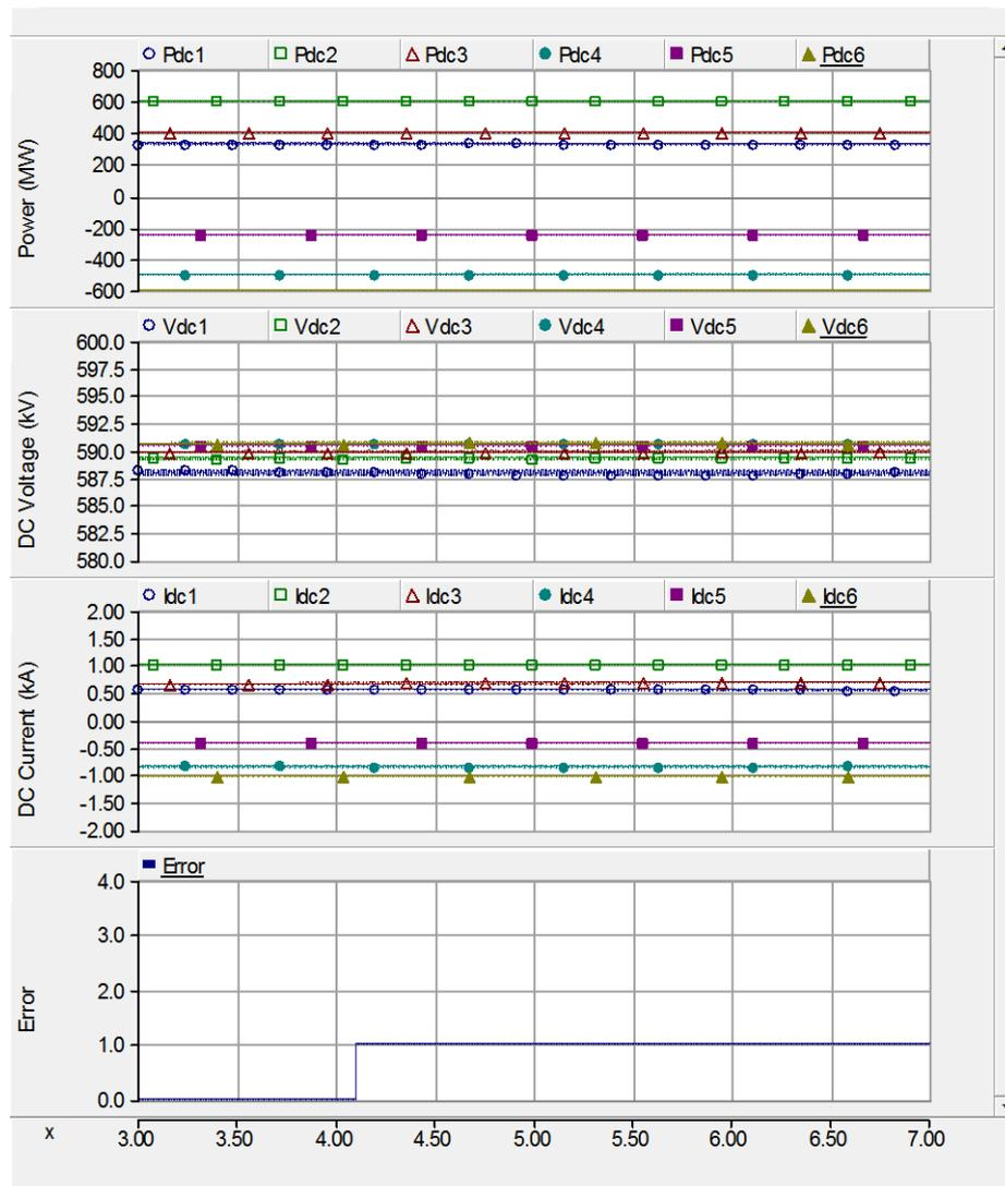
Figure 35: System's response to a DC power overload; x-axis is time in seconds.
