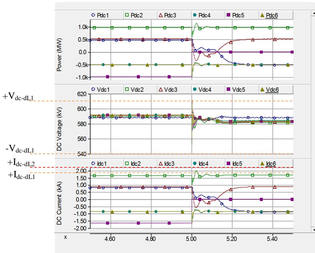
Figure 39: System's response to VSC5 being blocked at 5s; x-axis is time in seconds.
