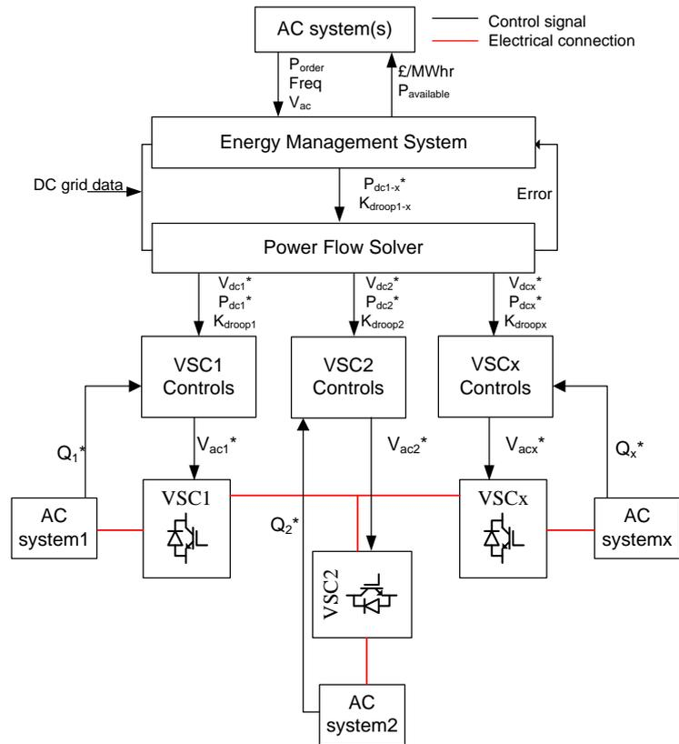
**Figure 1: Example DC Grid Control Architecture**
