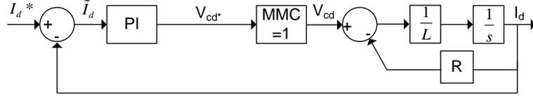
Figure 17: d-axis current loop without d-axis system voltage disturbance
