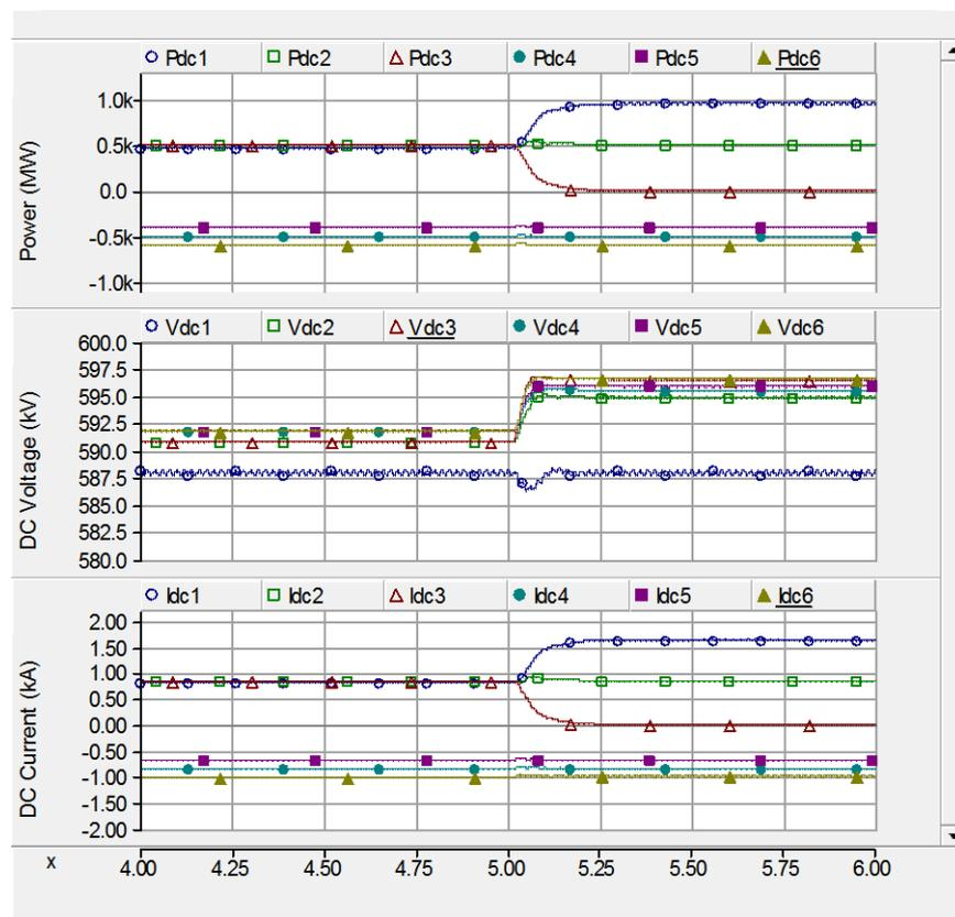
Figure 42: System's response to a power order increase for VSC3 from 500MW to 0MW at 5s when using the PFS; x-axis is time in seconds.
