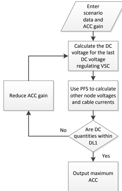
Figure 30: Flow chart for ACC gain algorithm
