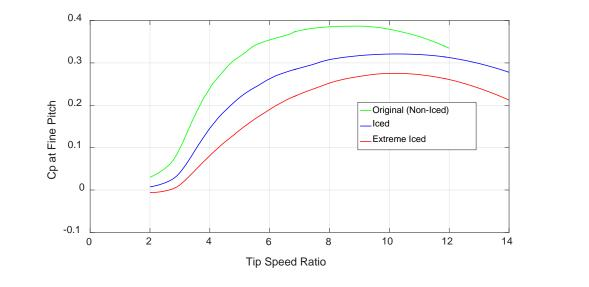
Under iced conditions the wind turbine will likely be stuck in the first constant speed section of the control strategy, and/or tracking a C<sub>p.max</sub> value it
