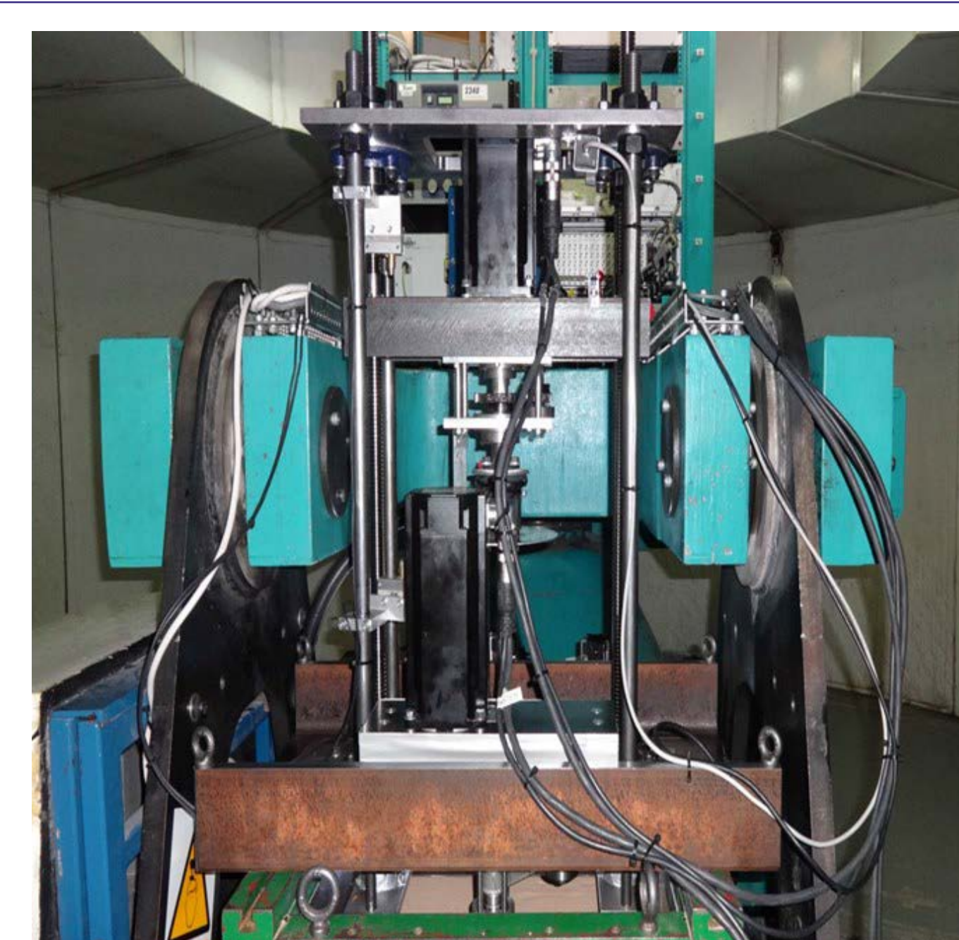
Figure 4. UoD centrifuge with screw pile installation & testing rig 3 .
