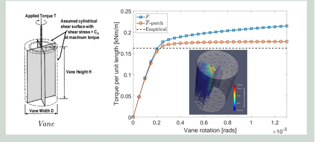
Example 2: the rotation of the partial screw-pile was simulated and the torque was computed. The torque from  $\mathbf{F}$ -patch method (MPM FBP) is more physically correct than from the standard MPM, because it is consistent to the material elasto-plasticity.
