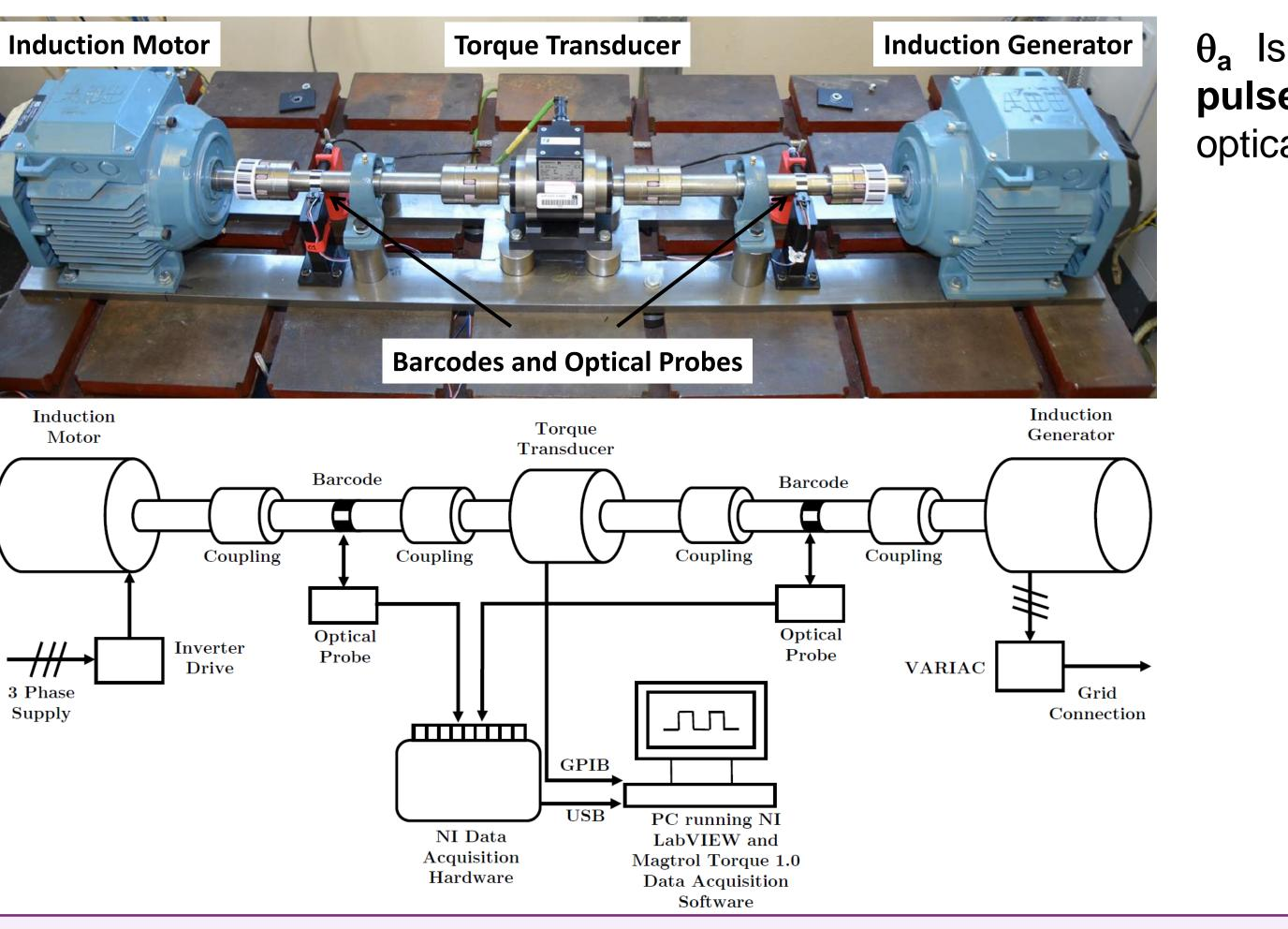
$\theta_a$  Is calculated from the phase shift,  $\Delta t$ , between pulse trains produced by two sets of bar codes and optical probes located along the shaft<sup>5</sup>
