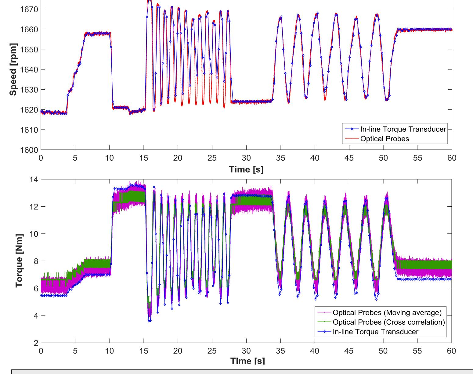
Speed (top) and torque (bottom) response under **transient** conditions due to smooth shaft torque variations between -2 and -10 Nm.
