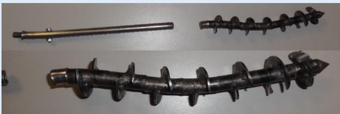
Fig.6: Screw pile damaged after penetration of 200 mm in the dense sand ( D_r 73%) at 50g.
