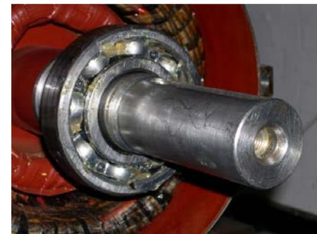
Generator outer race bearing fault - test rig
