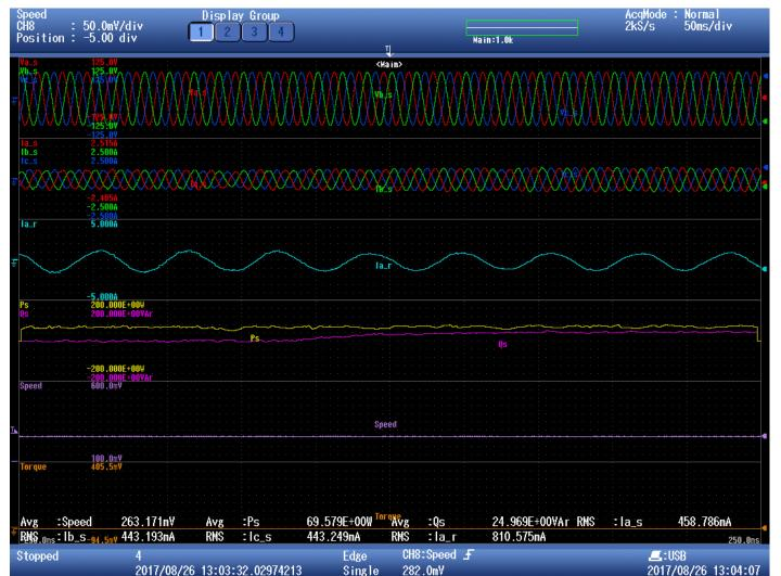
Reactive power can be controlled without affecting the machine speed.
