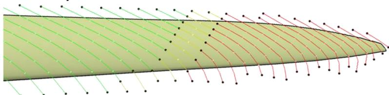
Figure 2 - Kinematic draping simulation results (red means  $>10^\circ$  reorientation)
