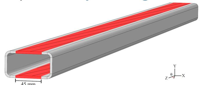
Figure 3 - Schematic of demonstrator highlighting flange regions in red
