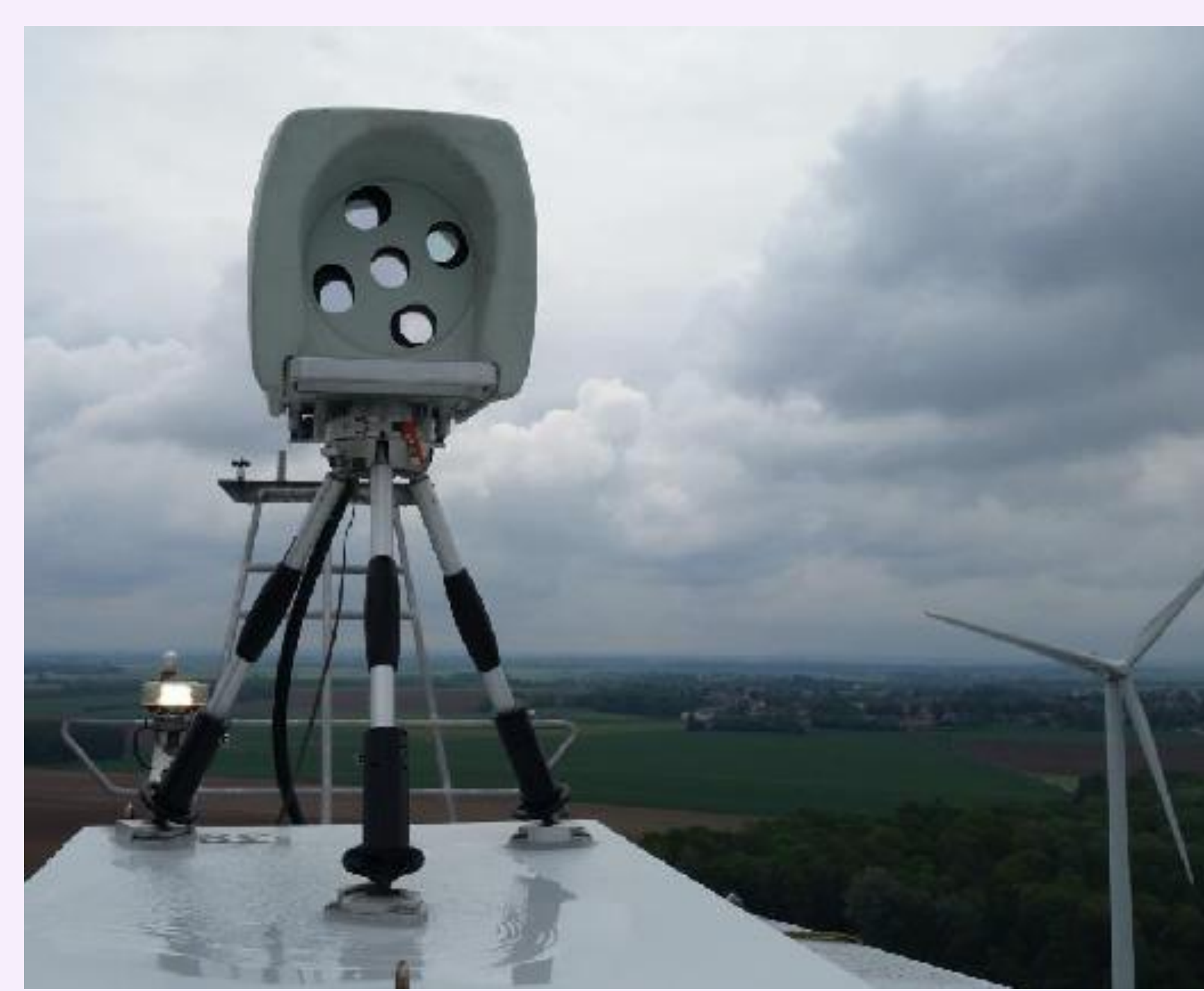
Figure 3: Leosphere 5 beam LiDAR mounted on top of the upstream turbine. The LiDAR can provide data with a frequency of up to 1Hz
