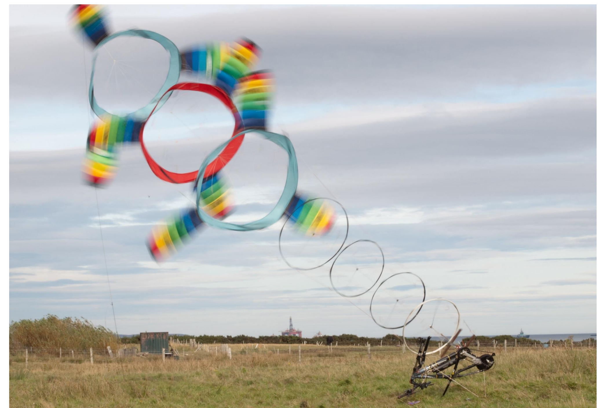
Daisy kite prototype undergoing testing on the Isle of Lewis. Photo taken by Rod Read, founder of Windswept and Interesting Ltd [5].
