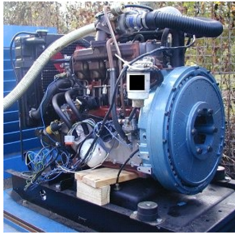
Pre production prototype permanent magnet generator developed at Durham School of
