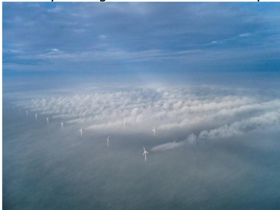
Fig. 4. Typical wake effects, which the Consortium are modelling, observed on a large offshore wind farm.
