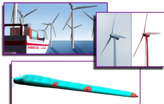
Fig. 8. Wind farm radar cross section (RCS) models developed by the Consortium.
