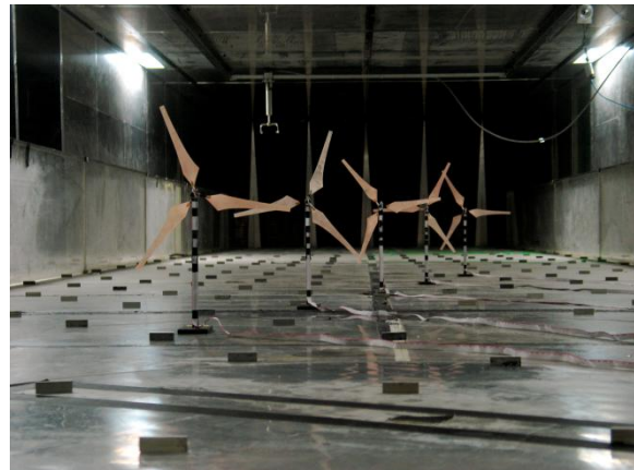
Fig. 5. Wind farm wake measurements being undertaken by the Consortium.
