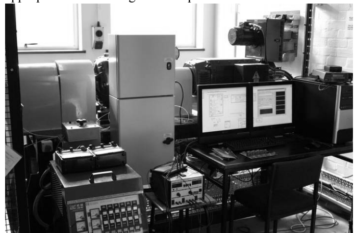
Fig. 3. Condition monitoring test rig and instrumentation showing generator (left), instrumentation (centre) and DC drive motor (right).
