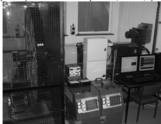
Fig. 3. The test rig, with the caged generator (left), driving DC motor (right).
