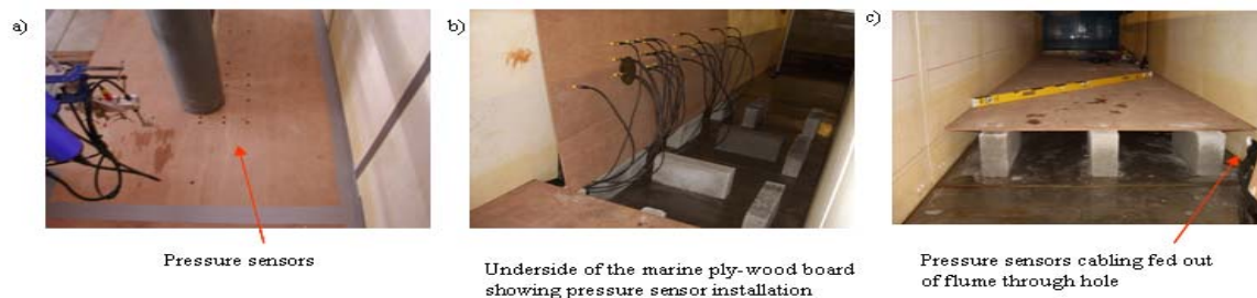
Figure 2-5 a-c. a) image from upstream of the pressure sensor pads embedded in the plywood board. c) image showing the underside of the board. c) image showing the hole in which the cabling is fed out of the flume
