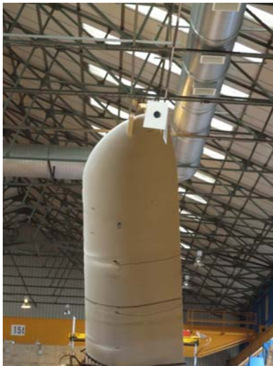
Figure 3: Target (black dot on white background) attached to tip of blade and digital camera used for tip-tracking of blade during dual-axis fatigue test.
